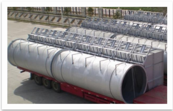
Flue gas conversion valve
